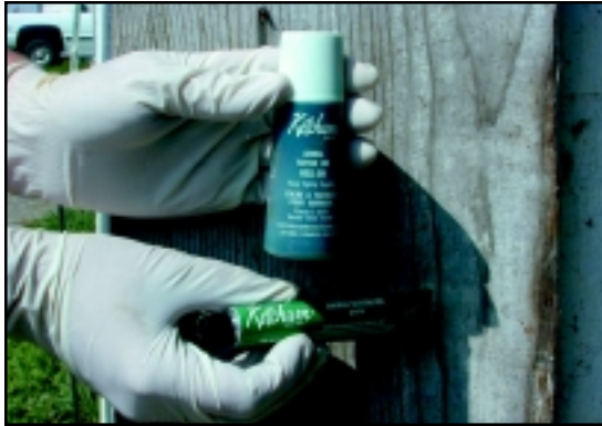
Two varieties of ink available are the roll-on (top) and the paste (bottom). The roll-on variety is most commonly used.
